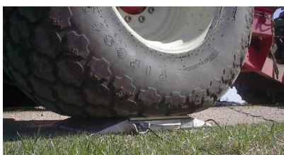
Figure 1. Weigh pad used to weigh a manure tank wagon.
