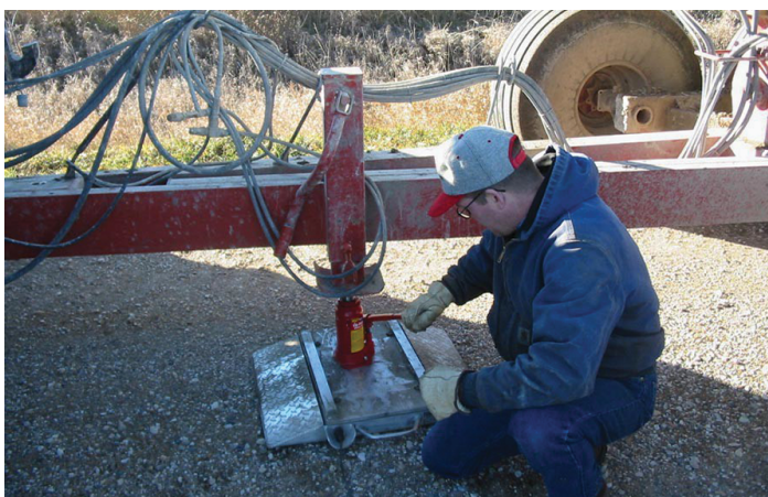
Figure 2. Weighing the hitch on a manure tank wagon.
