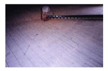
This is a sweep auger. It helps to collect grain when the bin is almost empty. Because it goes slowly in a circle on the floor, it can be an entanglement hazard to someone in the bin when it is operating.
