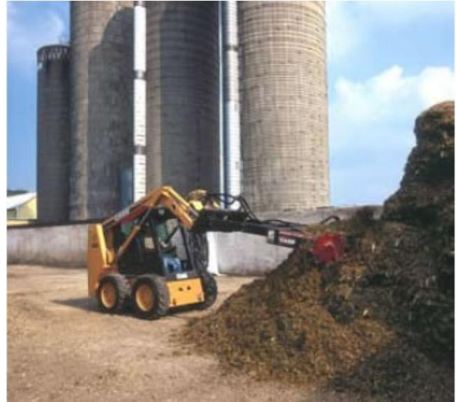
Figure 7. A defacer attachment on a skid steer or material handler boom helps break up silage over the entire face of the horizontal silo for safe removal of the silage.
